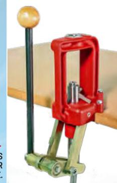
▶ SPENT PRIMERS COLLECTED AND DROPPED INTO FLEXIBLE PLASTIC TUBE FOR EASY EMPTYING.
