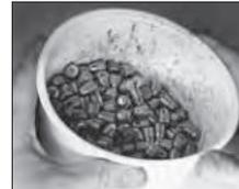
Gently shake bullets in an orbital motion to coat the bullets. If they do not coat completely, add a little more lube.
