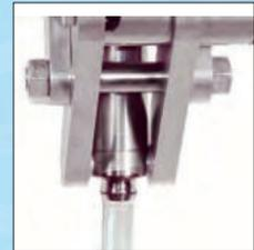
SPENT PRIMERS COLLECTED AND DROPPED INTO FLEXIBLE PLASTIC TUBE FOR EASY EMPTYING.
