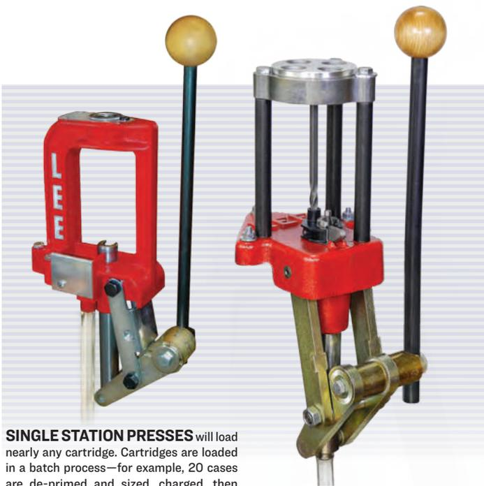
**SINGLE STATION PRESSES** will load nearly any cartridge. Cartridges are loaded in a batch process—for example, 20 cases are de-primed and sized, charged, then bullets seated. This die changing process is sped up by the Lee Breech Lock Quick-Change System. Rifle case reloading is best accomplished on a single station press. For a beginner, a single station press in a kit is the best value.
