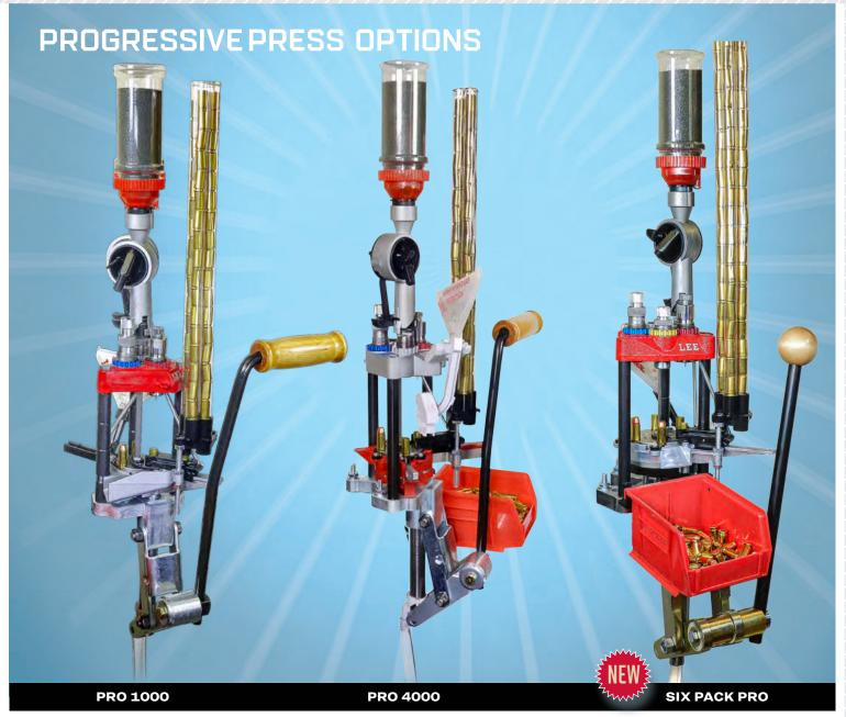
**2023 PRO 1000** Time proven design updated with rock solid tool head with Smart Lock quick change bushings. Improved tray fed primer feed, simple, reliable and safe with any brand primer. Simplified automatic indexing with no adjustments required. Add a bullet and pull the lever; other operations are automatic.
