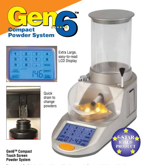
The compact Gen6 design takes a minimum of bench space and offers unrestricted pan and touch screen access for both right- and left-hand users. Accurate to one tenth grain, The Gen6 dispenses all types of smokeless powder at two grains per second. In addition, it features an auto repeat function that drops a precise charge each time the pan is reset.
